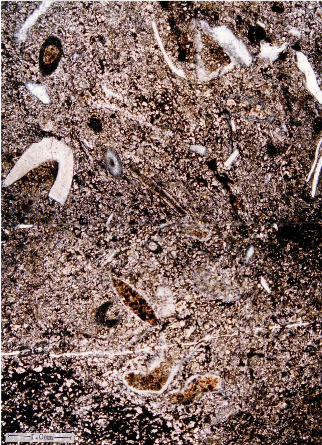
Plate 7.0: Photomicrograph of thin section DC 9 in P.P.L. showing bioclastic debris in impure limestones from Scoberry Bridge.
