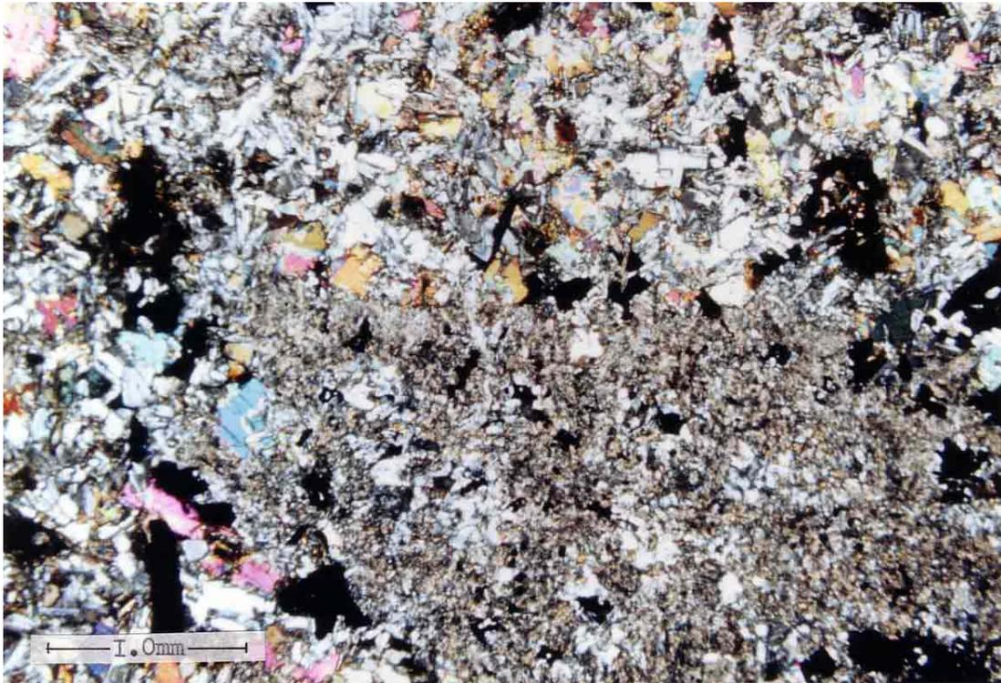
Plates 5.5: Photomicrograph of thin section DC 5, in X.P.L. showing patch of groundmass (Bottom right of picture).
