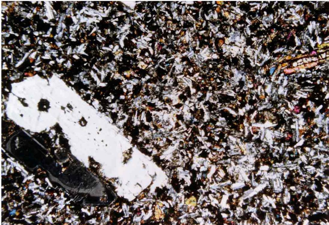
Plates 5.6, 5.7: Photomicrographs of thin section DC 6 in P.P.L. (top) and X.P.L. (bottom), showing porphyritic texture and zoning/twinning in plagioclase.
