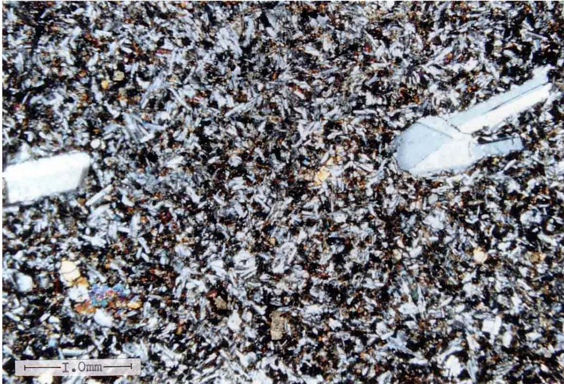
Plate 5.8: Photomicrograph of thin section DC 8, showing clusters of microphenocrysts enclosed by a fine grained intergranular, interstitial and sub-ophitic groundmass (X.P.L.).
