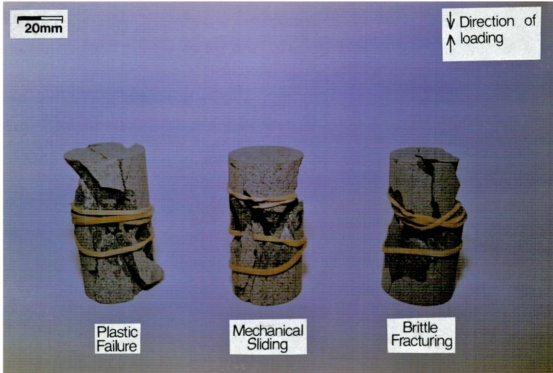
Plate 5.6. Sheared specimens of 38mm diameter Whin Sill dolerite.
