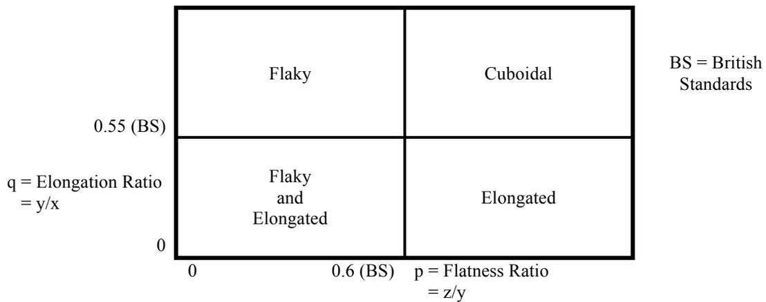
Figure 5.2. Aggregate Shape Measurements.
