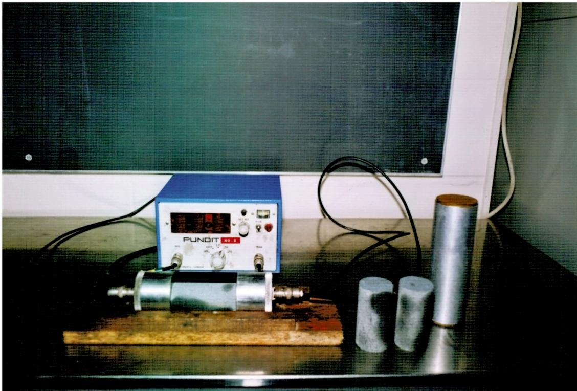
Plate 5.7. "Pundit" apparatus used for the determination of ultrasonic velocities.
