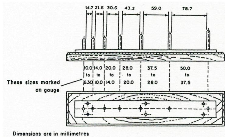
Figure 5.3. British Standard Length Gauge (BS812, 1975), after Collis and Fox (1985).
