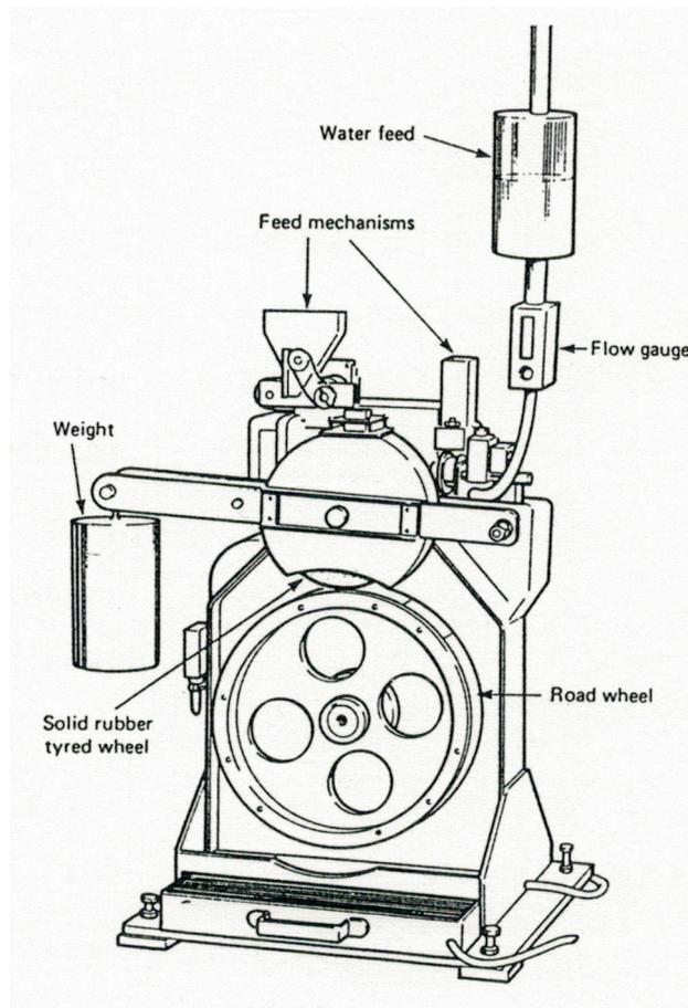
Figure 5.7. Accelerated polishing machine for conducting polished stone values. (Collis and Fox, 1993).
