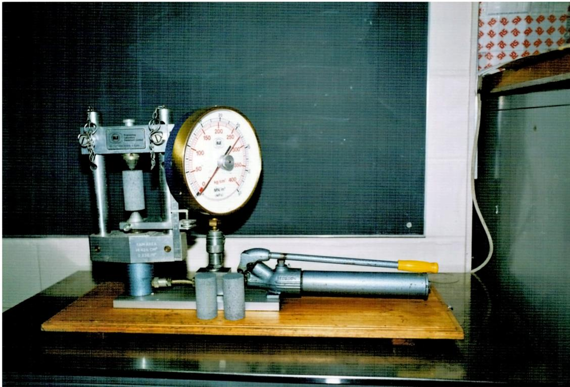
Plate 5.3. Franklin Point-Load Strength Apparatus.
