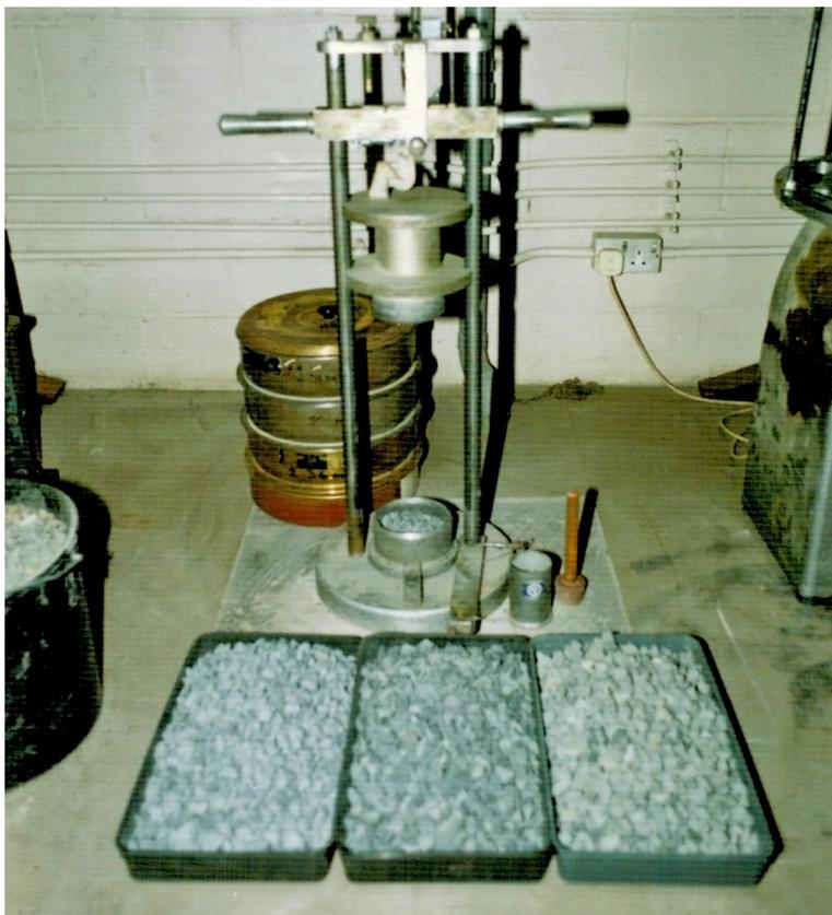
Plate 5.1. Aggregate Impact Value apparatus.
