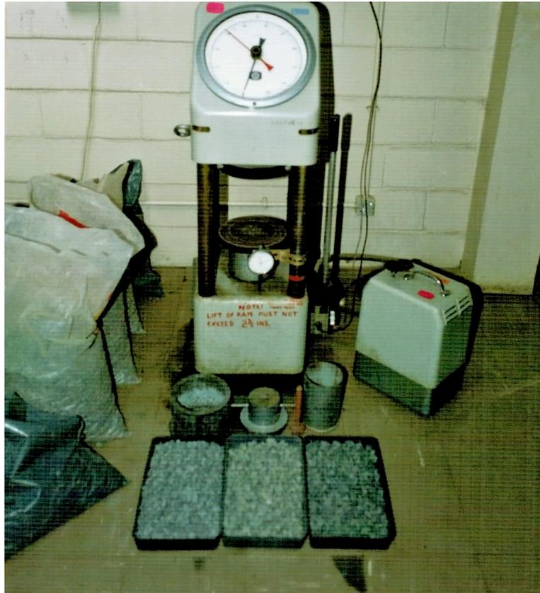
Plate 5.2. Aggregate Crushing Value and 10% Fines Value apparatus.
