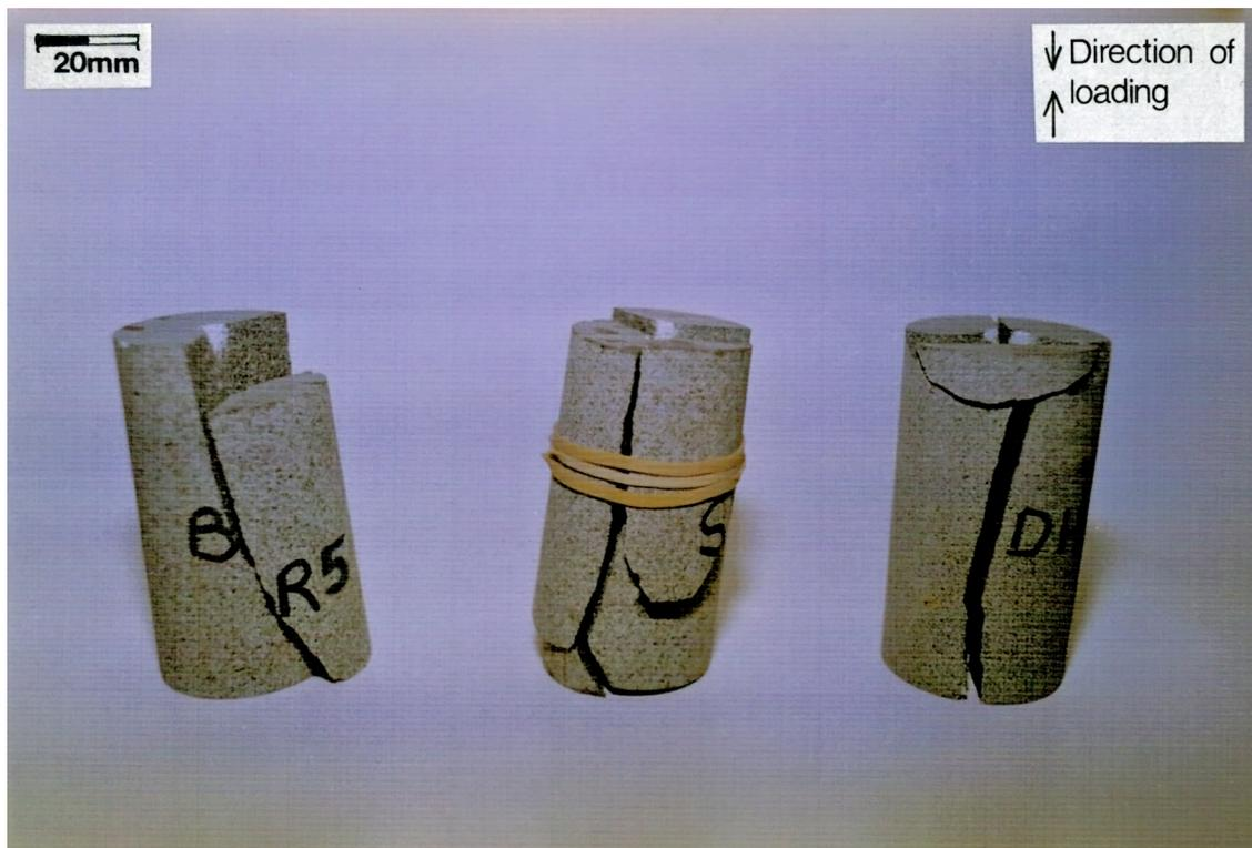
Plate 5.4. Tensile failure of Whin Sill dolerite cores.
