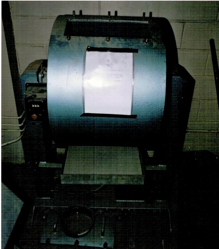
Plate 5.8. Los Angeles Abrasion Value test machine.
