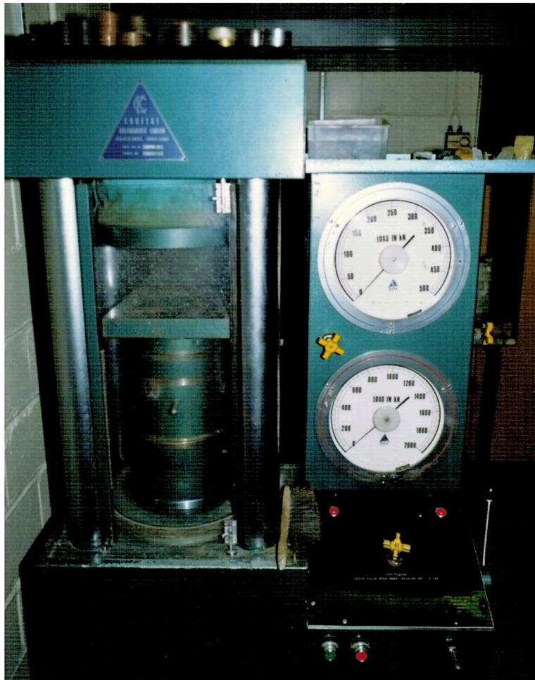
Plate 5.5. Equipment used to conduct Unconfined Compressive Strength Tests on Whin Sill dolerite.
