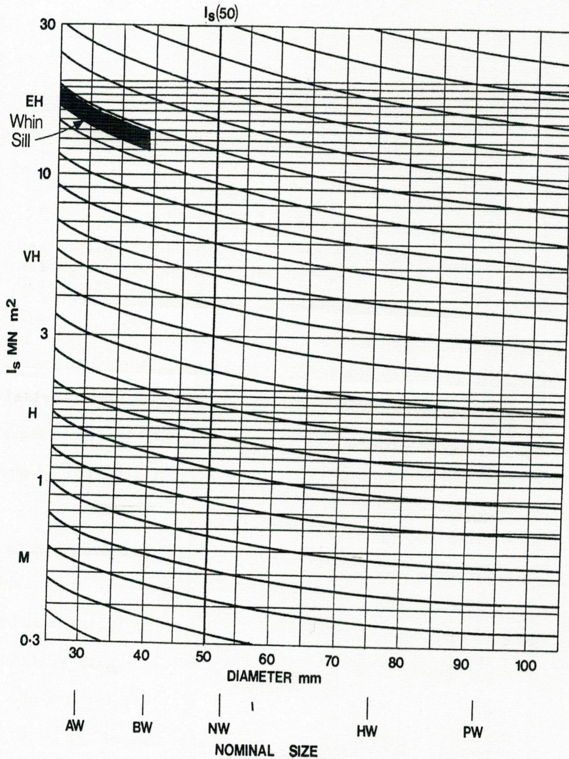
Figure 5.5. Point-Load Strength Correction Chart. (Brock and Franklin, 1972).
