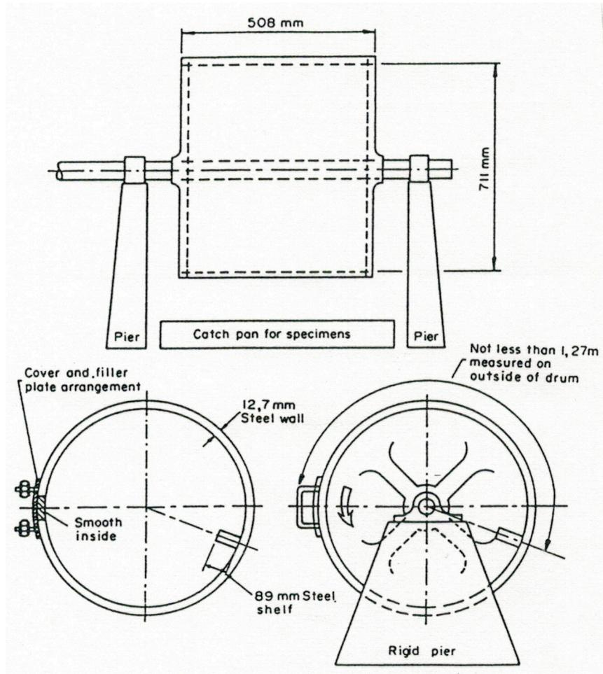
Figure 5.6. Los Angeles abrasion machine. (Collis and Fox, 1993).
