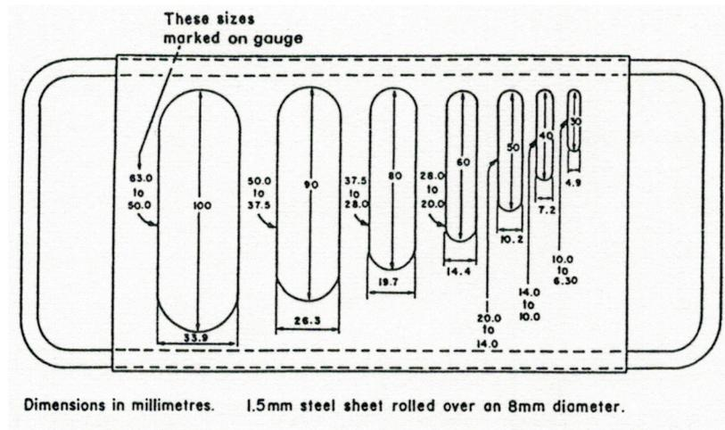
Figure 5.4. British Standard thickness gauges (BS812, 1975), after Collis and Fox (1985).
